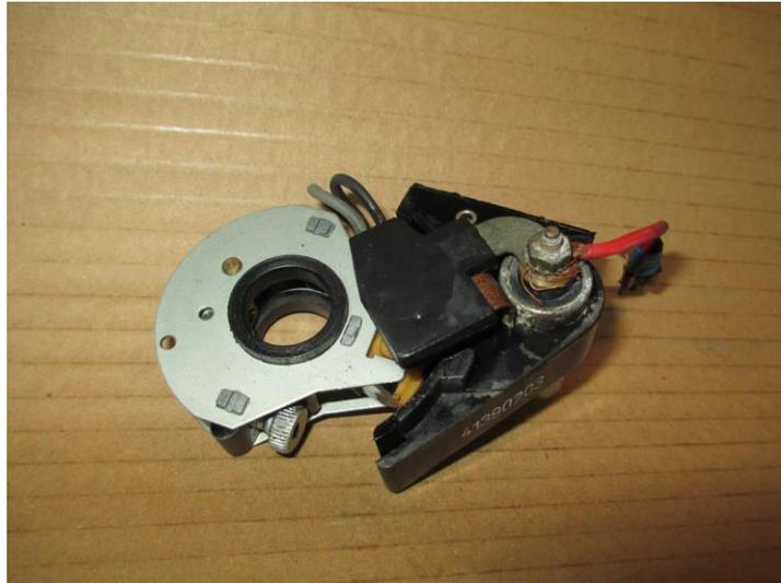
Once the new cassette and condenser are connected to each other, slip the condenser back into its holder and the cassette onto its spigots and slip the whole assembly back into the distributor and connect the earth wire to the bottom of the condenser. Connect your dwell meter (red lead to top of condenser or negative side of the coil and black lead to earth) and start the engine. Usually the points cassette is pre-adjusted enough to run the engine.
