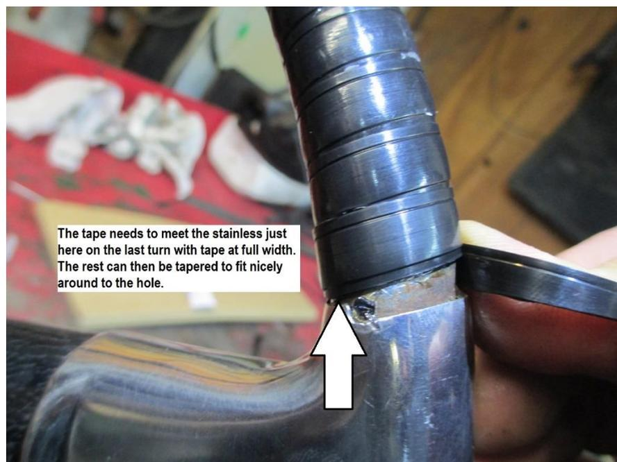
*Picture shows where the tape must meet the stainless. Notice how I had to overlap the last turns of tape less to make this happen. When the tape was overlapped fully, it left too large a gap at the end, but how yours works out depends on how much or little you overlapped it all the way around and how consistent you were.*
