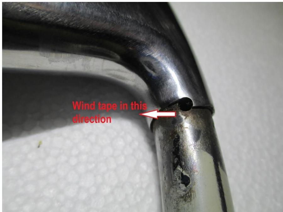
You now need to taper the starting end of the new tape so it looks like the end of the old tape you just removed, assuming at least one end was still intact! It is the overlapping side with the groove which must be trimmed off for a distance of 100mm, as in the diagram below. Cut along red line and discard bit marked with red crosses.
